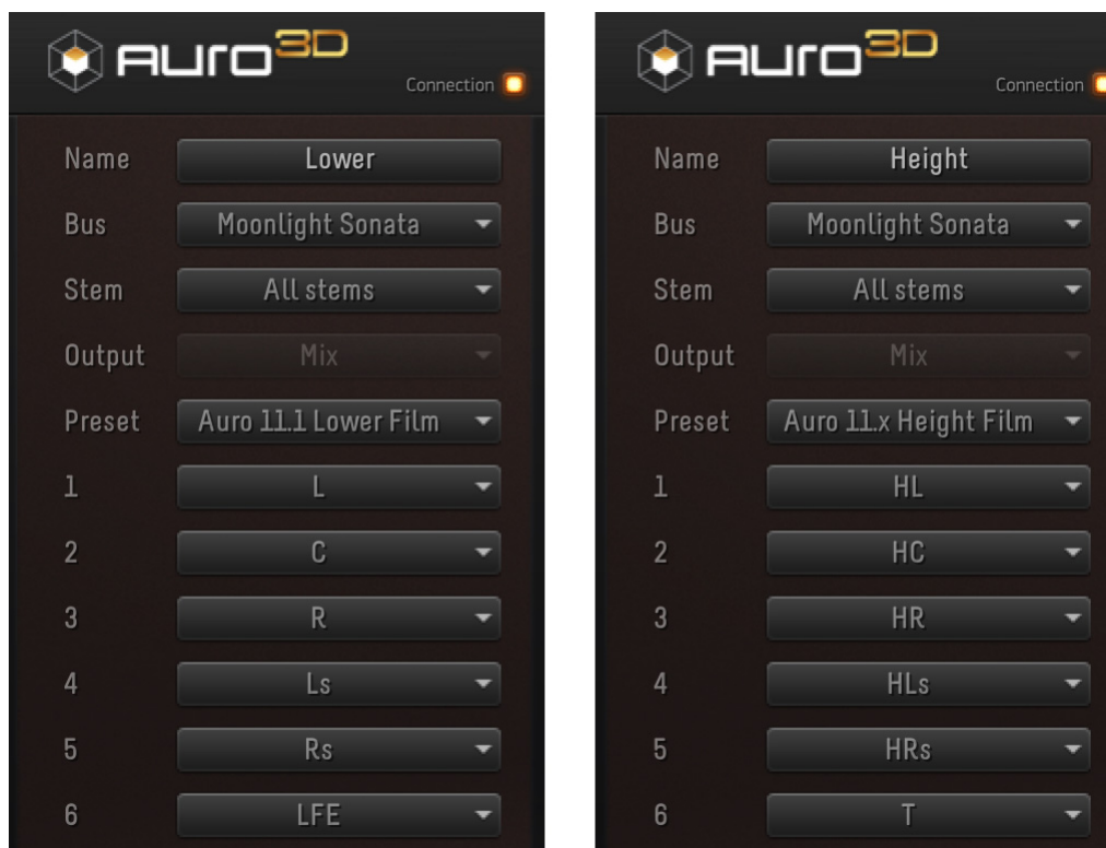
Figure 4-10 Two Auro>Returns deliver the output channels from Auro-Matic Pro 3D to the DAW.
